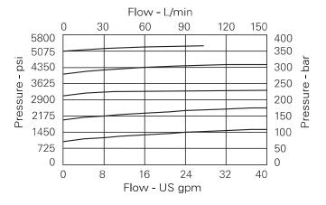
150 L/min (40 USgpm) 350 bar (5000 psi)
