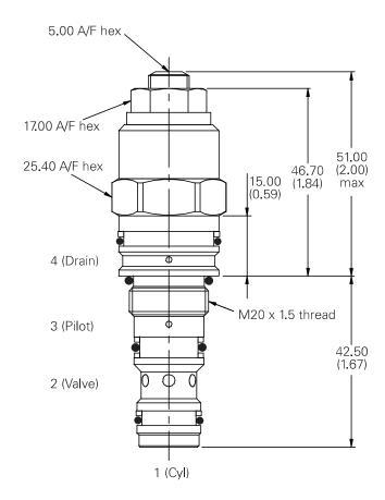
**Note:** Tightening torque of "F" adjuster locknut= 20-25 Nm.
